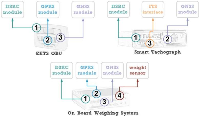
Figure 1 – Components of an EETS OBU, Smart Tachograph and OBW system
