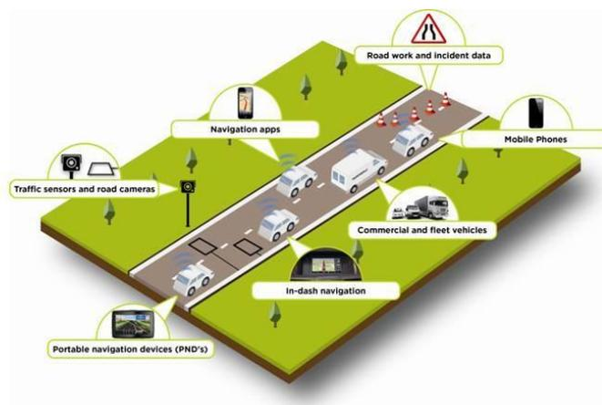
**Figure 4 – Data sources and transmission solutions from TomTom Traffic (PC Welt, 2015)**
